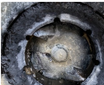
Grease build up in a grinder pump
