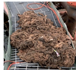
Wipes & Grease in a grinder pump
